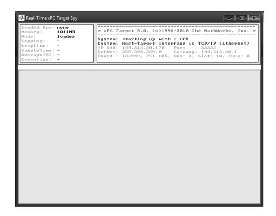
In the example above, the status window shows that the kernel is in loader mode and waiting to load a target application. 1 MB of memory is reserved for the application, 3 MB is used by the kernel, and 28 MB is available from a total of 32 MB. The xPC Target kernel uses the 28 MB for the heap, running scopes, and acquiring data.
